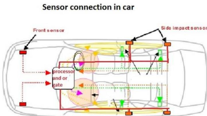
Figure: 5.1 Vibration Sensor connection in car
