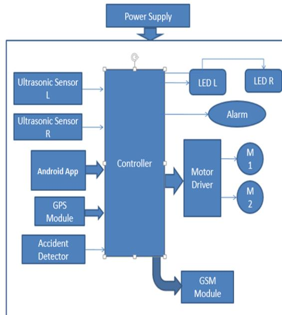
Figure 2.1. The block diagram of the system
